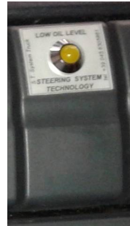
COD. 05256002 (YELLOW LED FOR MINIMUM OIL LEVEL OF STEERING SYSTEM)
