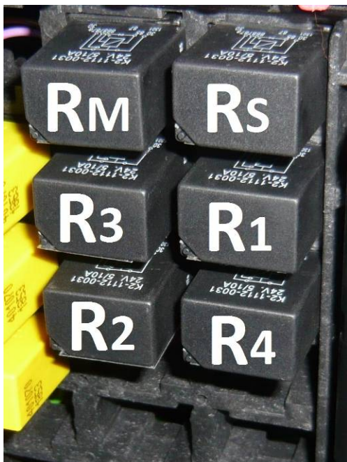
COD. 05255501 (RELAY' 24V-10A WITH DIODE)
